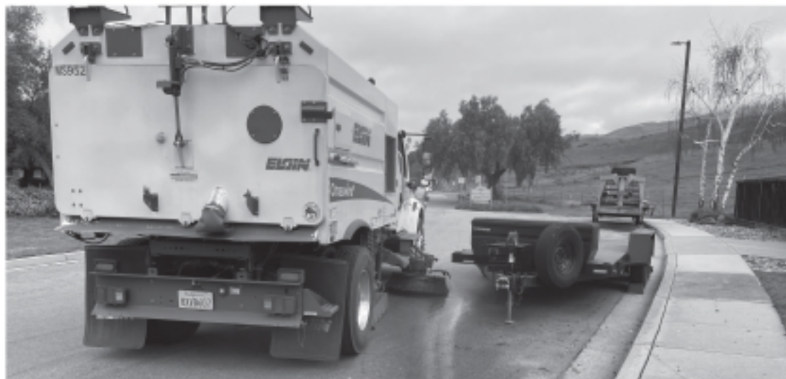
When vehicles and other obstructions block the street, sweepers cannot remove the litter against the curb.
